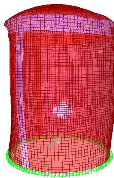
Figure 6: SAP-200 Model deformed shape against severe load combination
